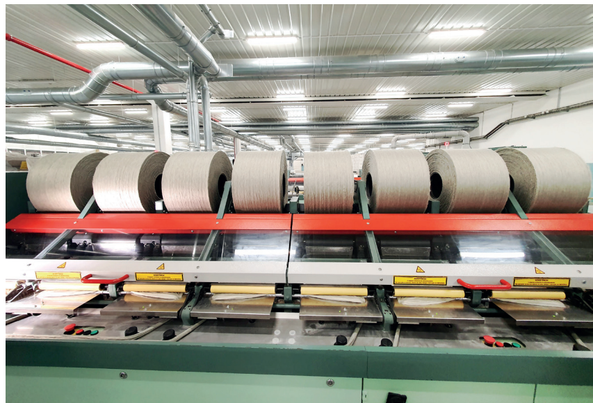
Fig. 30: The blend of virgin cotton and recycled fibers is processed on the comb at Portuguese customer Polopiqué.
